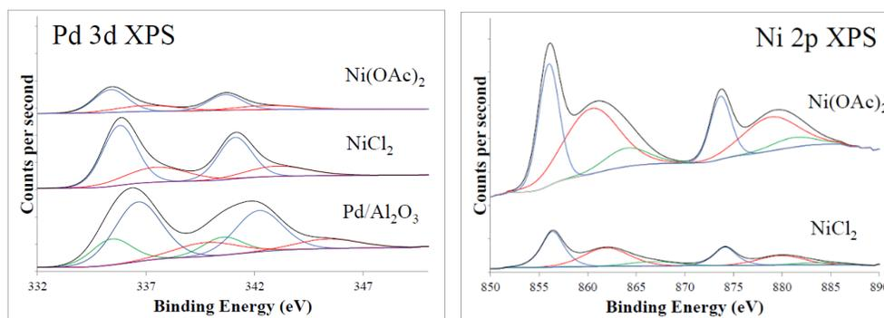
**Figure 1:** Pd 3d (left) and Ni 2p (right) XPS spectra for fresh Pd/Al<sub>2</sub>O<sub>3</sub> catalyst and spent catalyst after reaction with NiCl<sub>2</sub> and Ni(OAc)<sub>2</sub>
