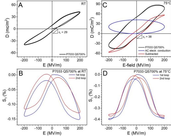
**Fig. 2.** Simultaneous measurements of (A,C) two continuous bipolar D-E and (B,D) longitudinal strain ( $S_1$ ) loops for the QS700% P7033 sample at 200 MV/m at (A,B) room temperature and (C,D) 75 °C, respectively. For D-E loops, subtraction of AC electronic conduction (shown as the blue horizontal loops) from the experimental data (black loops) results in neat ferroelectric loops (red loops).
