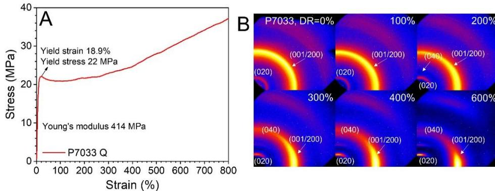
**Fig. 1.** (A) Stress-strain curve for quenched (Q) P7033 sample. (B) Corresponding 2D WAXD patterns during in-situ uniaxial stretching of Q P7033 at room temperature. The stretching direction is vertical.
