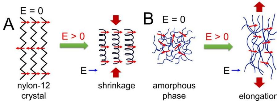
**Fig. 3.** Schematic models of (A) crystalline phase and (B) amorphous phase in uniaxially stretched PEBAX films upon the application of a high electric field. The stretching direction is vertical and the electric field is along the normal direction (the blue arrow) of the stretched film. Small red arrows represent the amide groups.
