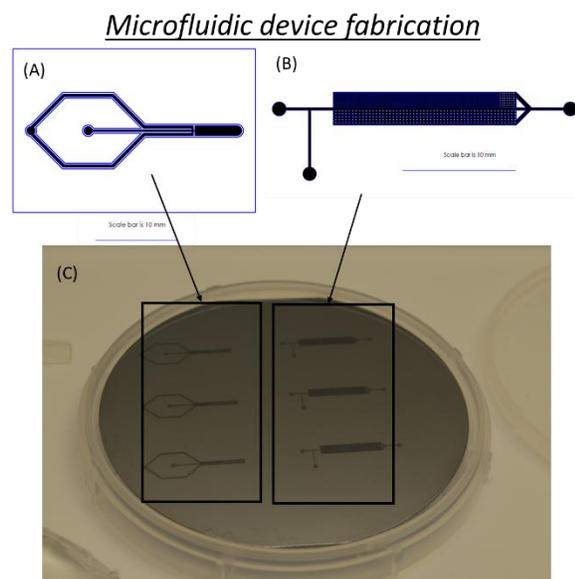
**Figure 1:** Microfluidic mold for fabricating PDMS devices for studying foams in porous media. (A) Tip streaming device design for generating foam, (B) Porous media design, and (C) mold for microfluidic device fabrication.
