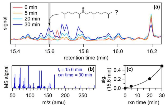
**Fig 3.** (a) Gas chromatogram of products formed when a pristane film is exposed to gas-phase hydroxyl radicals over a period of 30 minutes. (b) Mass spectrum of the shaded peak in the chromatogram, which may correspond to a ketone. (c) Exponential fit to the change in signal of the highlighted peak to model first-order kinetics.
