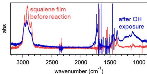
Fig 2. ATR spectra of squalene film before (red) and after (blue) exposure to hydroxyl radicals.
