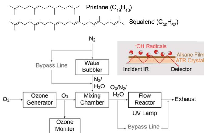
Fig 1. Flow assembly with ATR setup (inset). Adapted from references 4-5.
