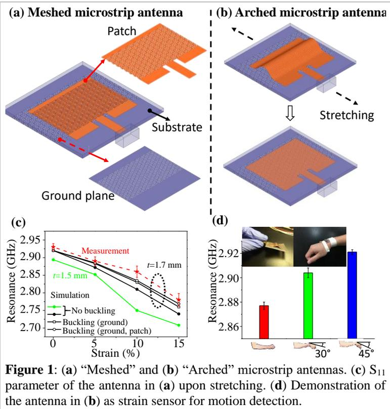
**Figure 1:** (a) “Meshed” and (b) “Arched” microstrip antennas. (c)  $S_{11}$  parameter of the antenna in (a) upon stretching. (d) Demonstration of the antenna in (b) as strain sensor for motion detection.
