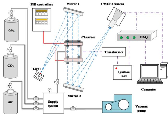
It was experimentally observed that the laminar burning speed increases with unburned gas temperature and the increase in pressure has an inverse effect on the laminar burning speed. It was also seen that with the rise in CO<sub>2</sub> concentration, the laminar burning speed decreases. A change in CO<sub>2</sub> concentration from 0% to 80% decreases the laminar burning speed non-linearly, consequently, a change in CO<sub>2</sub> concentration from 0% - 10% reduces the laminar
