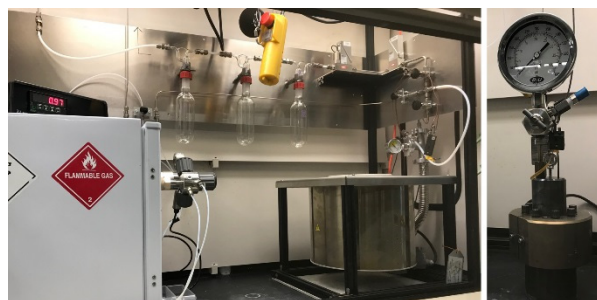
Figure 4. High-temperature (800 °C), high-pressure (34 bar) reactor compatible with H_2 evolution and air-sensitive gaseous precursors. Version 2.0 (with metal-metal seal) is commissioned as of Sep. 2019.
