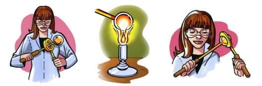
When heated, the atoms in the ball and ring vibrate faster. This increased motion competes with the attractions the atoms have for one another, so they move a little further apart. As the atoms move slightly further apart, the metal ball gets a little bigger.
