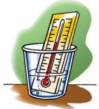
b. Why does the red liquid move down the tube when a thermometer is cooled? When cooled, the molecules in the liquid inside the thermometer get a little closer together. Because the liquid takes up less space, the red line moves down in the tube. If two thermometers have different liquids in them, the liquids can move to different heights in the thermometers even if they are measuring the same temperature. Why does that happen?
