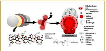
Schematic representation of the charge process. The active particle on the right side represents a hypothetical charge on a particle. While charging, electrons and Li ions leave the active particles. While ions accumulate at the surface with the plasticizer, the electrons are transported through the carbon and current collector to the external circuit.
