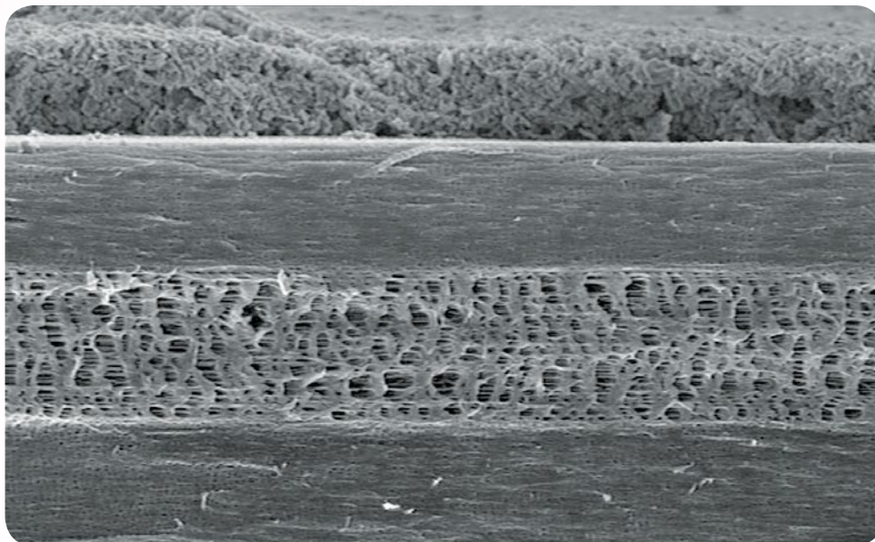
Cross-section SEM image of a ceramic-coated separator. The scale is about 30 μm from left to right.
