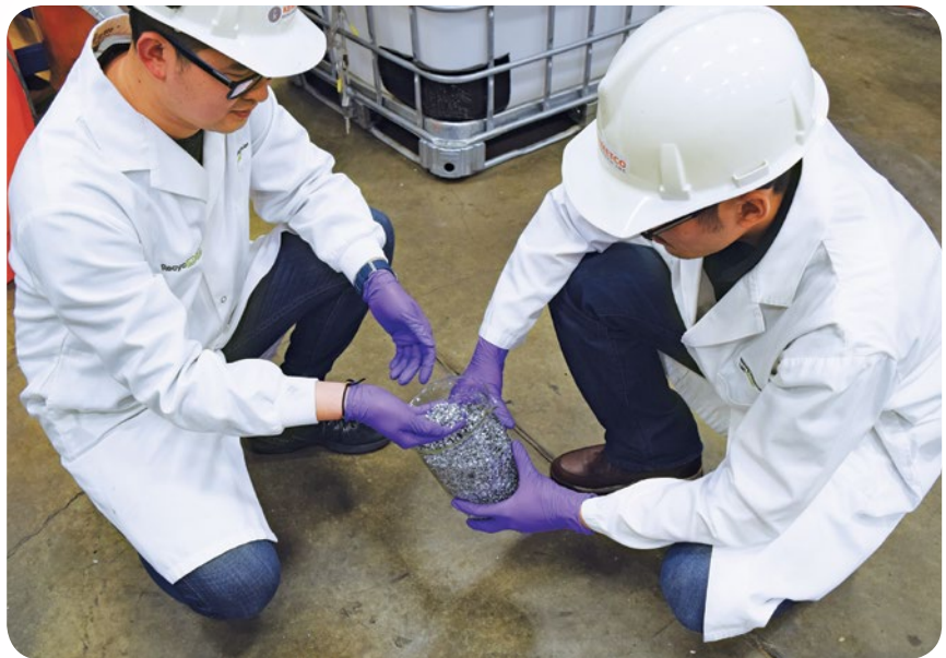
In a battery-recycling pilot plant near Vancouver, British Columbia, American Manganese engineers examine shredded aluminum recovered from Li-ion battery cathodes.
