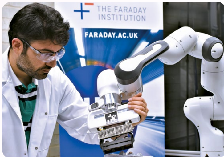
At the University of Birmingham, ReLib team member Alireza Rastegarpanah develops robotic methods for safe, automated processing of spent Li-ion batteries.
